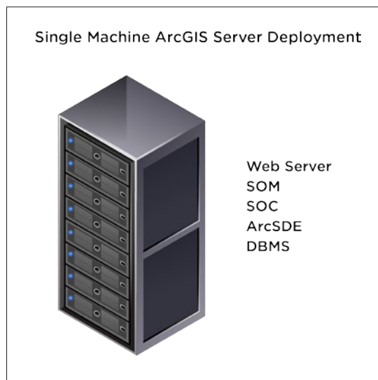
Figure 3. Single Machine ArcGIS Server Deployment
